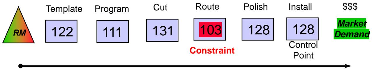
Clearly, in this example *Route* is the constraint of the system. It is the weakest link in the chain. Increasing the capacity at any other location will not increase the capacity of the system. This is the one place the company should focus on to increase overall system capacity.
